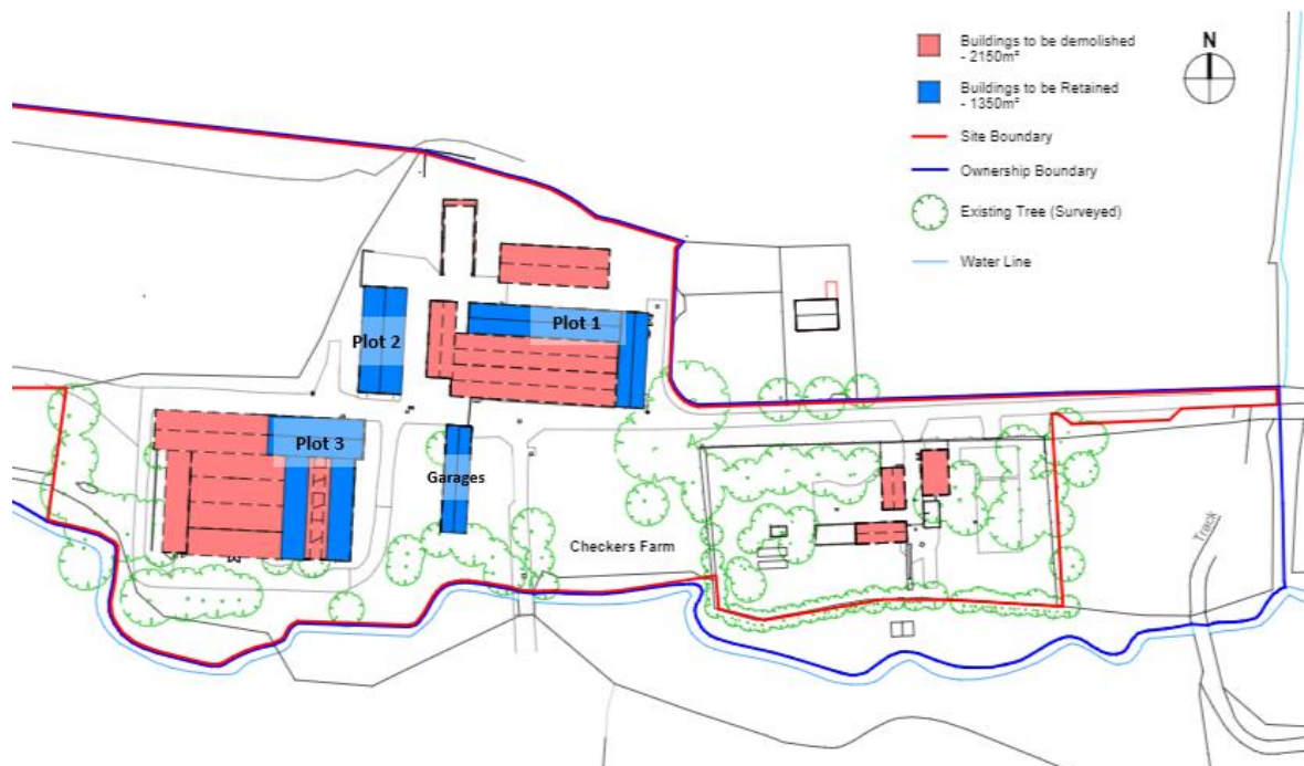
Fig. 2 - Extract of Demolition and Retention Plan
