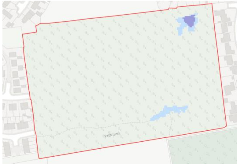
Extract from Flood Mapping showing Flood Zone 1 and Surface Water Flood Risk
